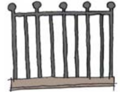
Metal railings on stone plinth up to 1m high when used at front. Up to 2m to side and rear.
